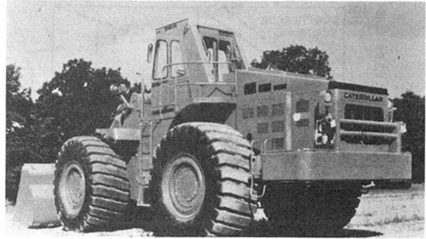
Fig. 5 Turbine-powered model 992 loader
